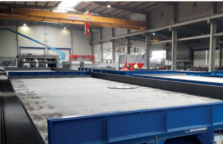
One of the Konecranes indoor cranes at the Avermann production line at Zbych-Pol & Mobet Sp. z o.o. is designed to pick up and transport a concrete spreader with stabilizer.
