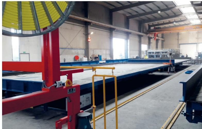
Avermann also delivered a device to smoothen the surfaces of the precast elements on the tilting tables (see foreground left).
