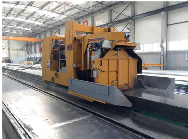
*Multi-angular cutting saw while cutting deep 500 mm hollow core slabs*
