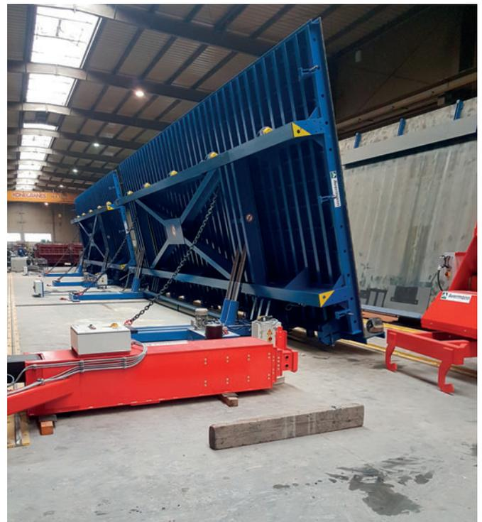
*Eight high-quality hydraulic tilting tables with a size of 13 x 4.5 m each have been installed at Zbych-Pol & Mobet Sp. z o.o.*
