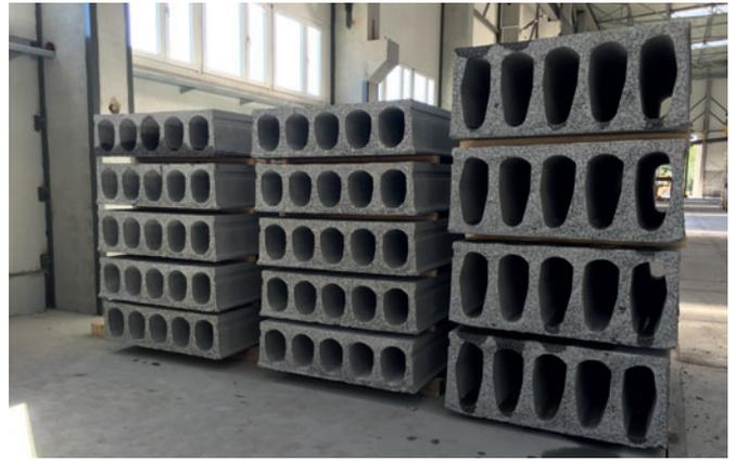
High quality hollow core slabs produced by Nordimpianti Extruder EVO machine
