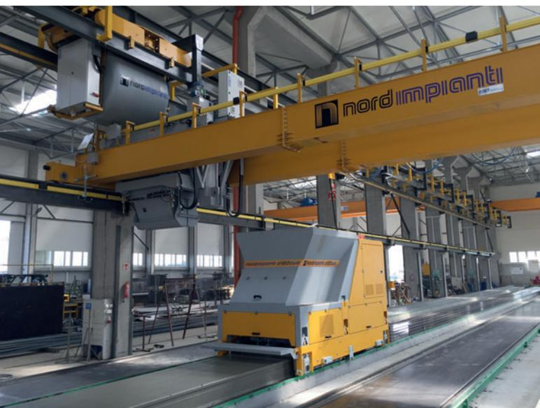
*Extruder EVO casting machine with fully automatic concrete distribution system*
