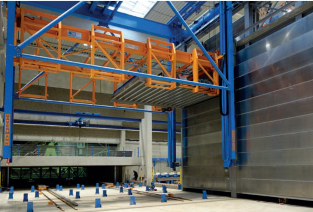
Storage and retrieval machine for hardening chamber feeding
