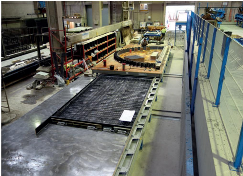
Fig. 5: Shuttering and reinforcing stations for solid/sandwich walls and custom elements
