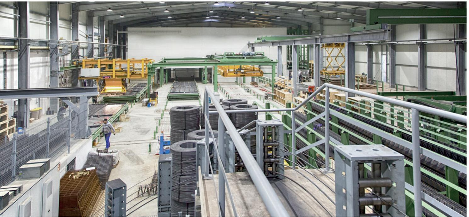
*Circulation plant – concreting/compaction area, turning and lifting station*
