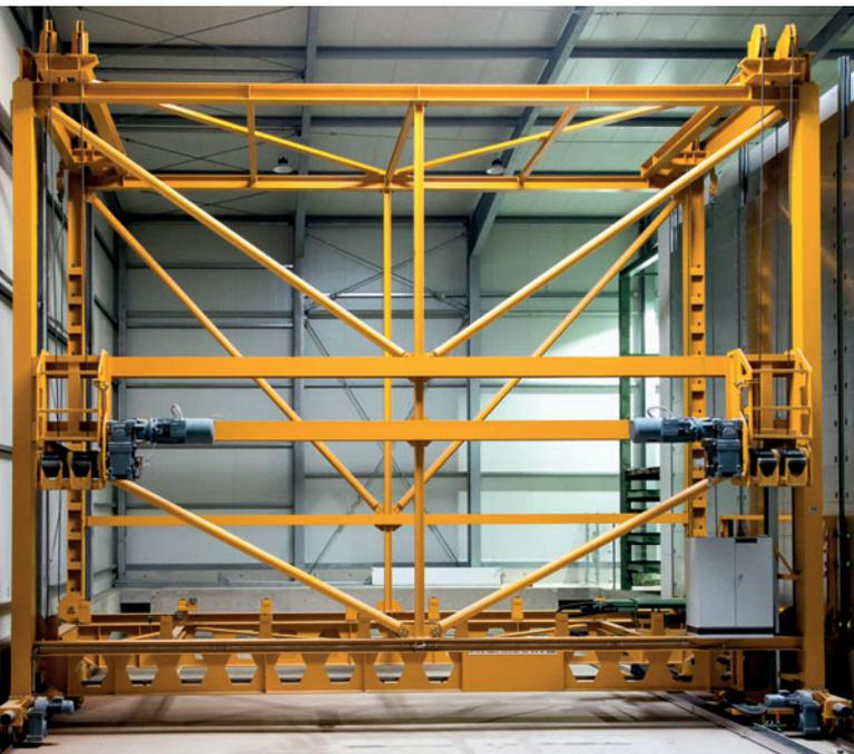
*Storage and retrieval machine for feeding the curing chamber*
