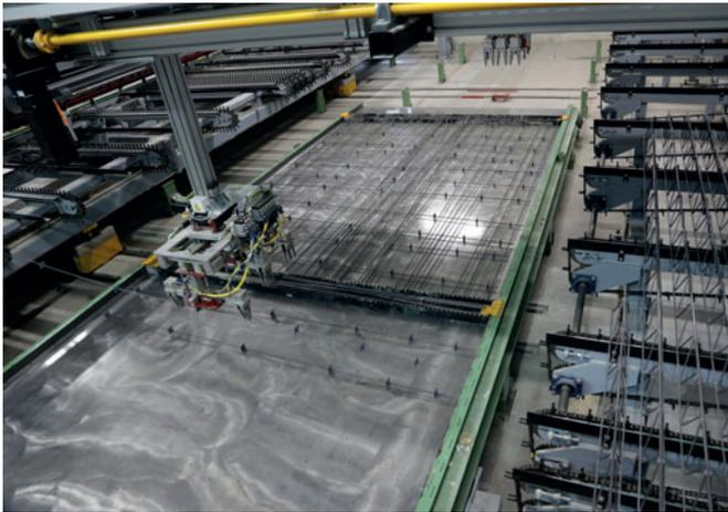
Fully automatic reinforcement plant with robot system from EVG
