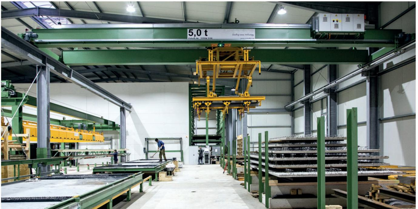
Special crane for lifting out the floor slabs
