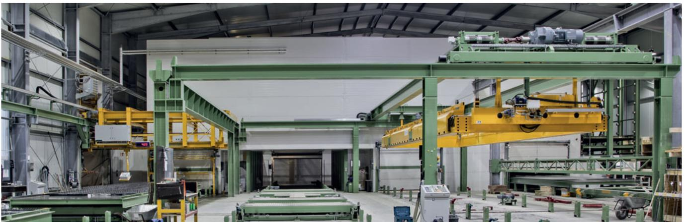
Vibrating compactors under the concreting station and the tilting table machine
