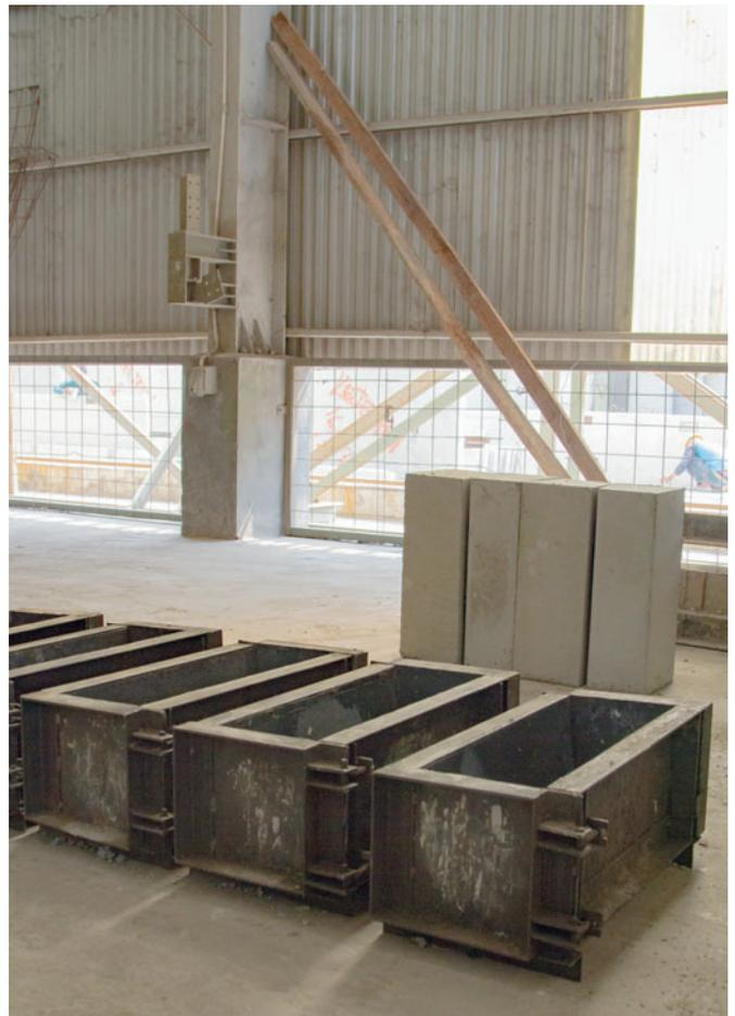
*Residual concrete is utilised by PT Motive Mulia for a by-product - kerbstones (at the rear) - that separate pavements from the road carriageway in the capital, Jakarta. The company makes its own steel moulds (in the foreground) for this purpose.*
