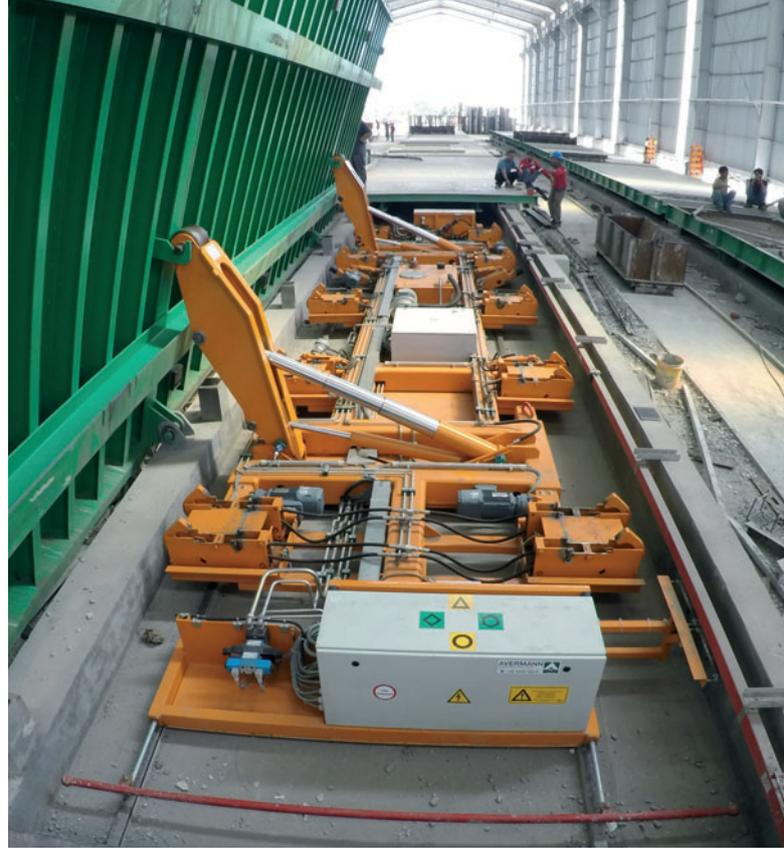
*The tilting-compacting machine's hydraulic device tilts the table on its pivot points up to an angle of 80° so that the hall crane can hoist finished wall panels undamaged from the formwork table.*
