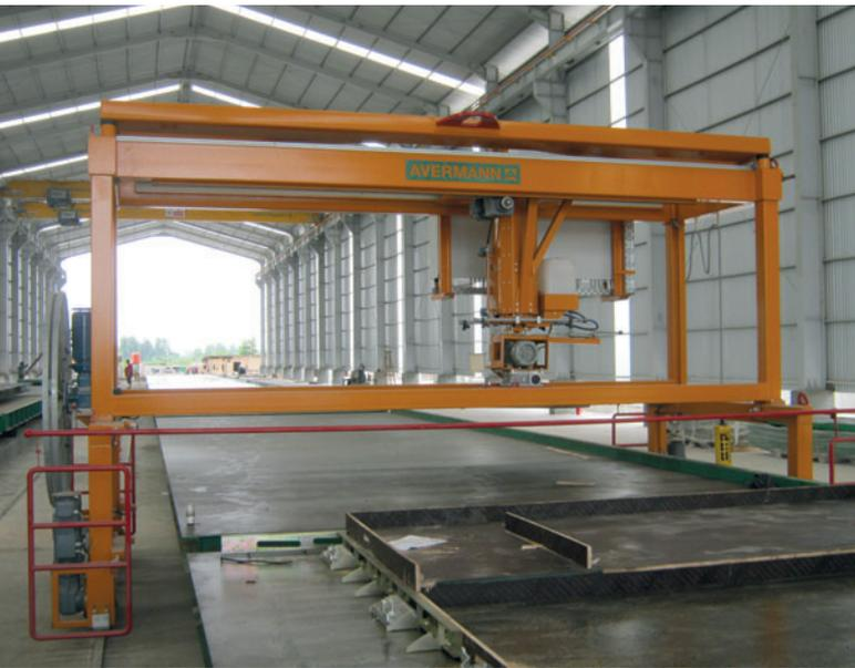
*The tilting table system includes this power trowel, which gives the necessary high quality to the rear sides of these flat precast concrete elements*
