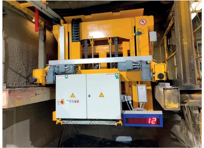
Travelling with each concrete spreader bucket are a control unit cabinet and digital weight measuring system with large screen display
