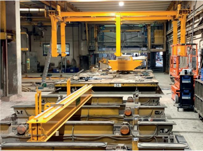
*The assembly had to be carried out just using manual means, such as chain hoists and heavy-duty rollers, without the aid of a hall crane*
