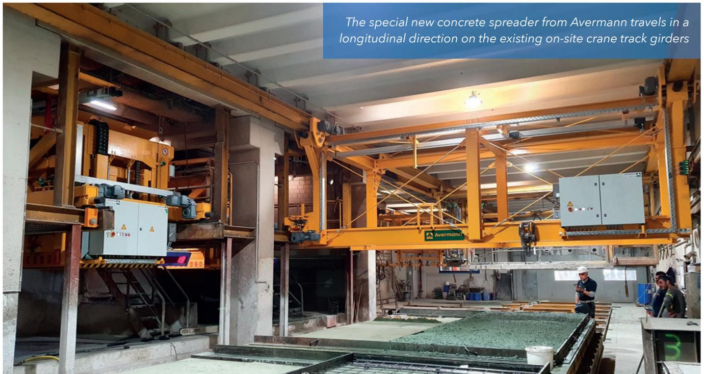
*The special new concrete spreader from Avermann travels in a longitudinal direction on the existing on-site crane track girders*
