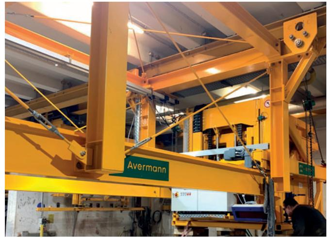
*The hoisting height of each of the two concreting buckets is about 1,100 mm*
