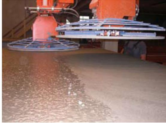
**Fig. 5** A pan-type wing float from Avermann smooths the surfaces of the precast parts after obstructing form parts were removed.
