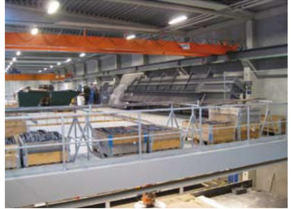
**Fig. 3** The reinforcement works are carried out on the mezzanine floor of the hall. The completed mesh reinforcement and cages are lowered into the formwork from above.
