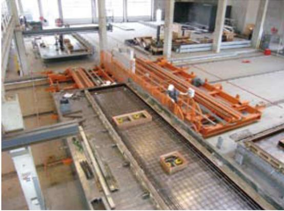
**Fig. 4** The sliding unit for shifting the pallets.
