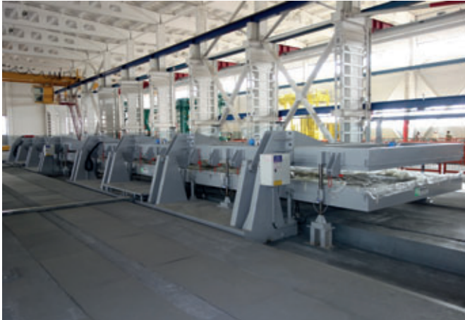
Folding pallets for the production of double walls and lattice girder slabs
