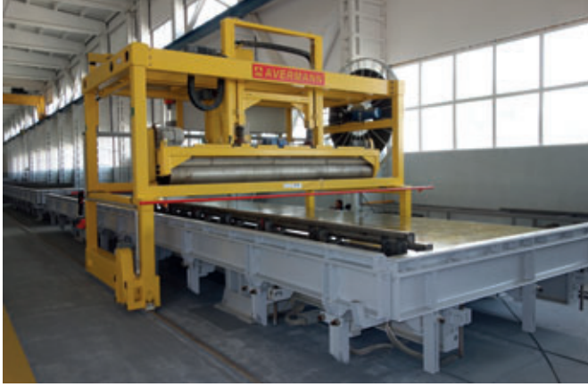
View inside one of the two production halls with tilting tables and smoothing machine
