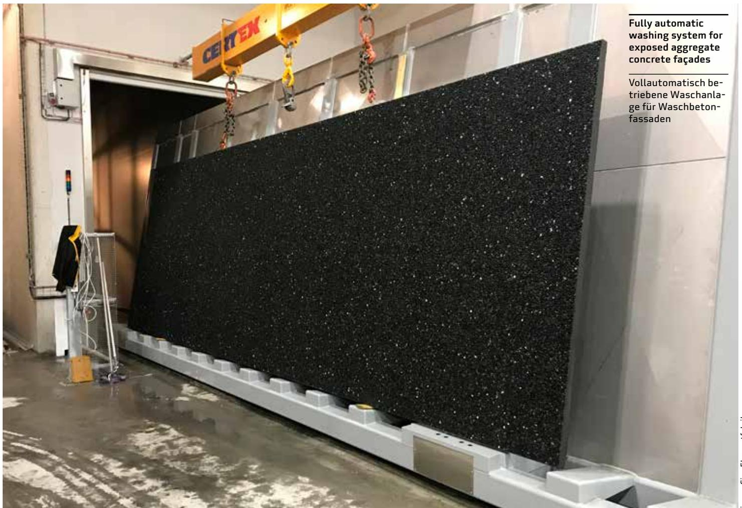
Fully automatic washing system for exposed aggregate concrete façades
