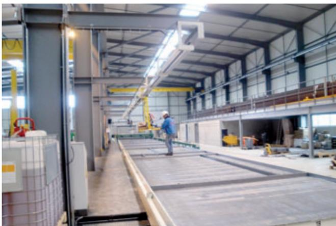
Manual formwork bays with work station system
