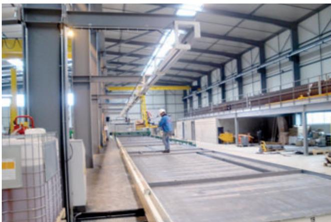
Manual formwork bays with work station system
