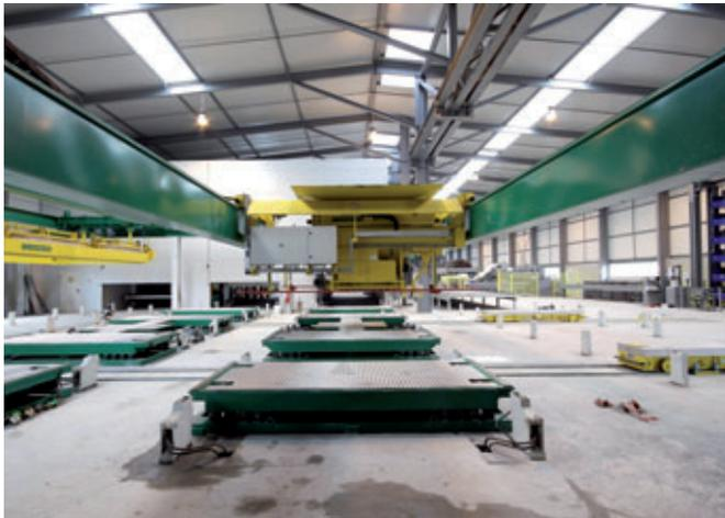
Vibratory compactor and concreting bay with concrete spreader
